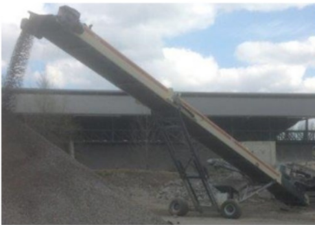
MC1050-24W 24m Wheel Conveyor x 1050mm Wide Belt
